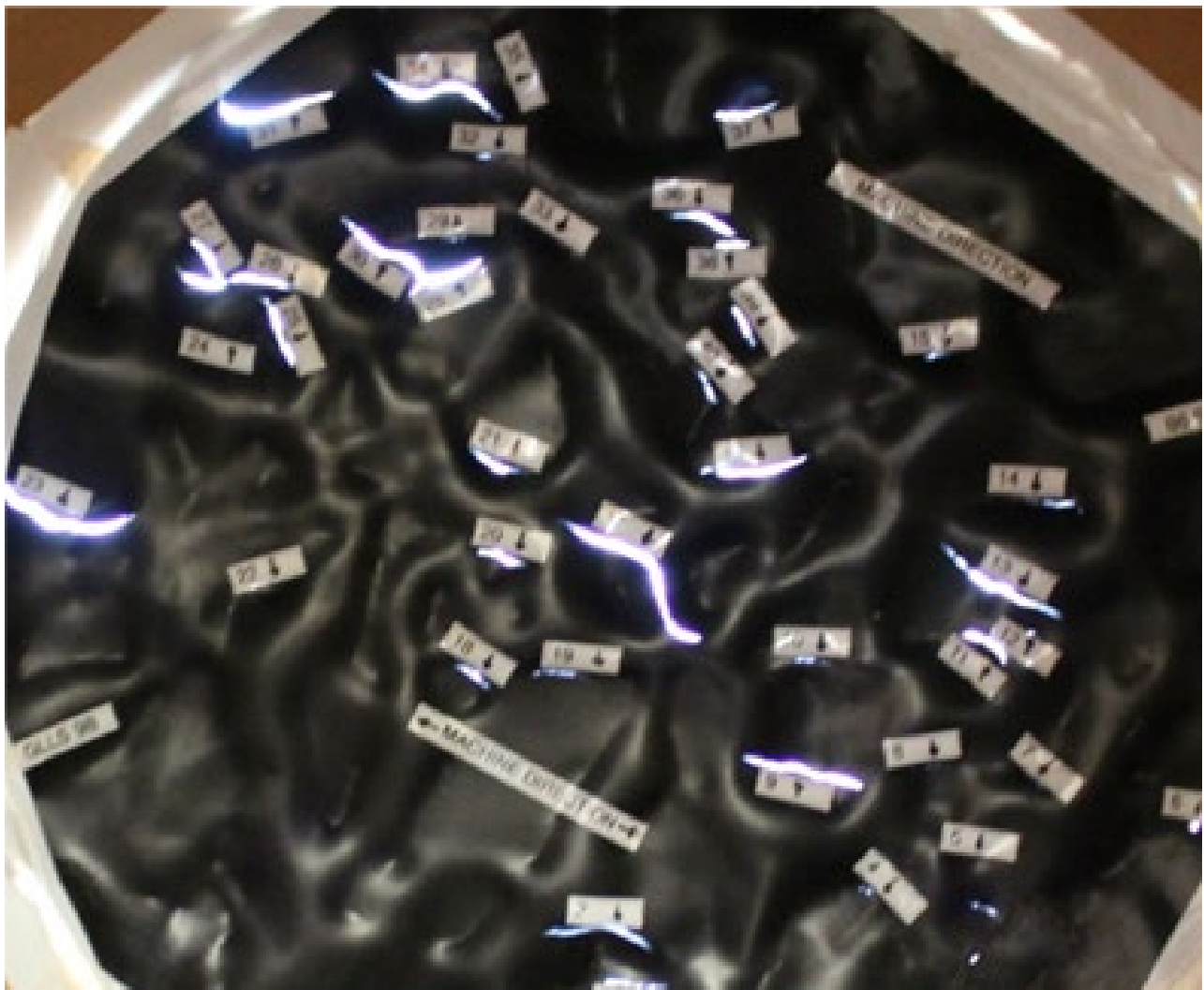
Figure 7: End of Service life for HDPE GMB. 0.6 m diameter specimen under 250 kPa of pressure with 61 (2014)
